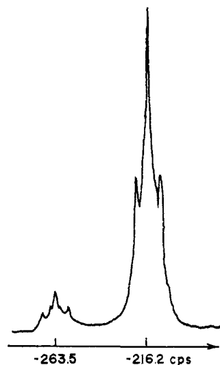
Figure 3. Proton magnetic resonance spectrum of the \alpha -hydrogens of tetrahydrofuran in a solution of dichloroborane in tetrahydrofuran at 28^\circ .
